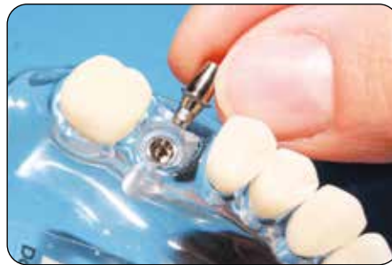
2: Depending on gingival height you can either scan the abutment base or use a scanpost (art no. C-030-00052). In cases with high gingiva a scanpost is preferable.
