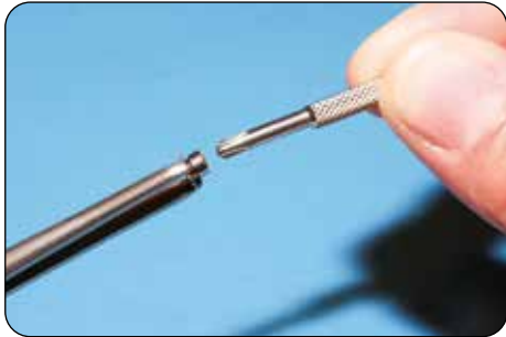
7: Adjustment of the retention with the activator.
